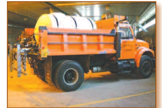
A salt brine solution dispensed from this truck will help keep Upper Milford roads passable this winter season.
